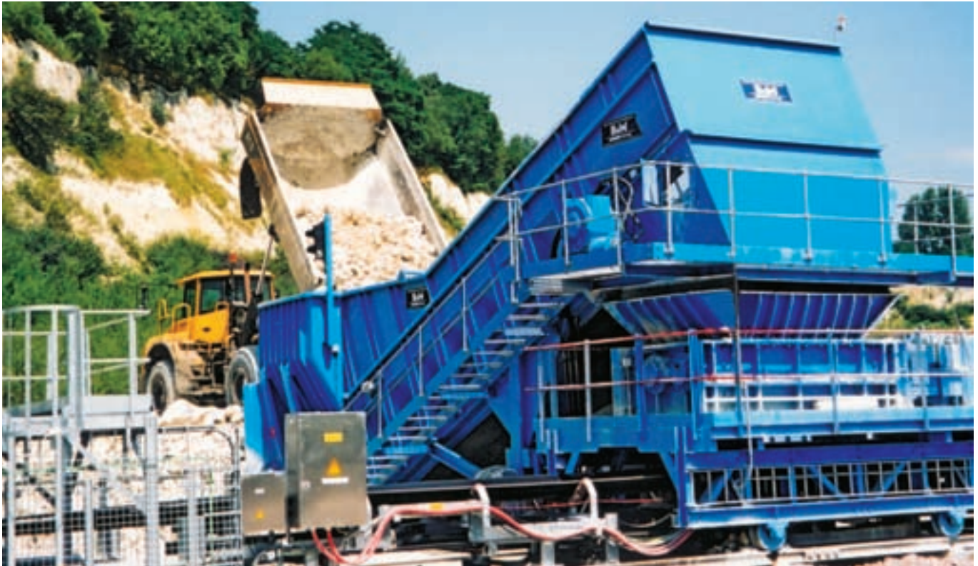
SAMSON™ plus Twin Shaft Rotary Sizer receives as-mined Limestone from dump trucks and provides a manageable lump size for onward conveying
