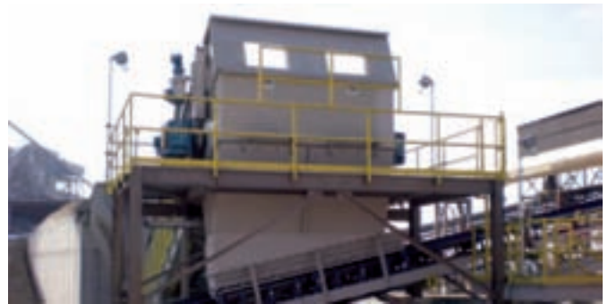
SAMSON™ 1600 with Tandem Drives using two Helical/Bevel Speed Reducers mounted one each side of the extended head shaft
