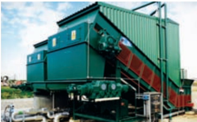
Twin Screws meter output to Progressive Cavity Pump
