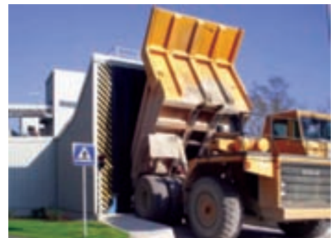
SAMSON™ plus Twin Shaft Rotary Sizer receives as-mined Limestone from dump trucks and provides a manageable lump size for onward conveying
