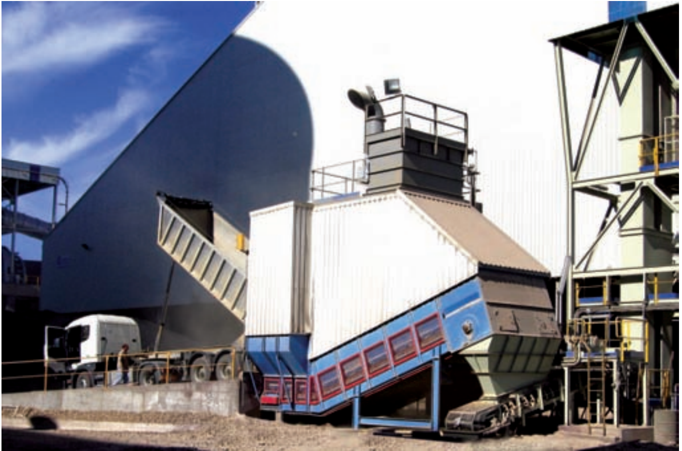
The SAMSON™ with Deflected Chassis and Full Enclosure including Dust Filter receives Cement Clinker
