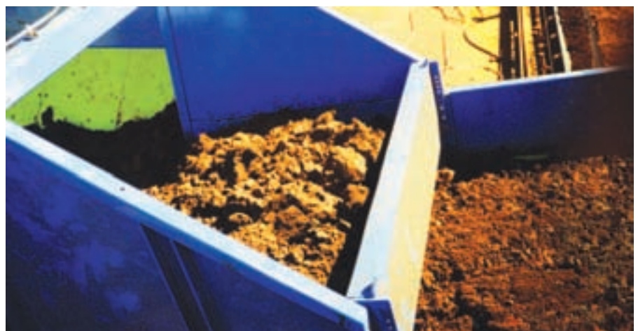
Levelling Blade controls the material bed depth at the SAMSON™ Discharge
