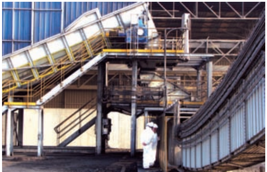
SAMSON™ supplied with Vibrating Screen to remove oversize material before onward conveying
