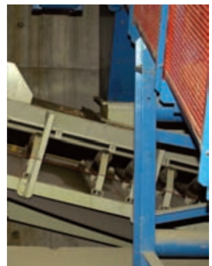
The Wide Apron-Belt SAMSON™ Concept permits a Shallow Excavation and Economical Installation
