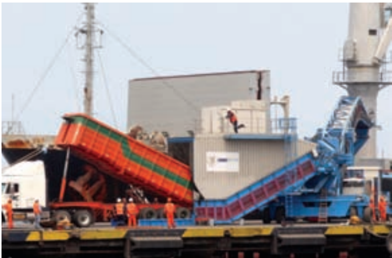
SAMSON™ Feeder integrated to a Mobile Shiploader receives Copper and Gold Concentrate
