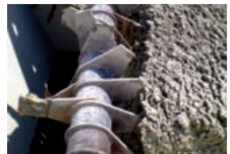
Rotating Teaser provides a closely controlled discharge rate handling wet clay
