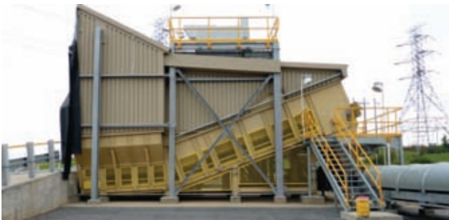
SAMSON™ Raised Discharge permits transfer direct to surface mounted belt conveyor
