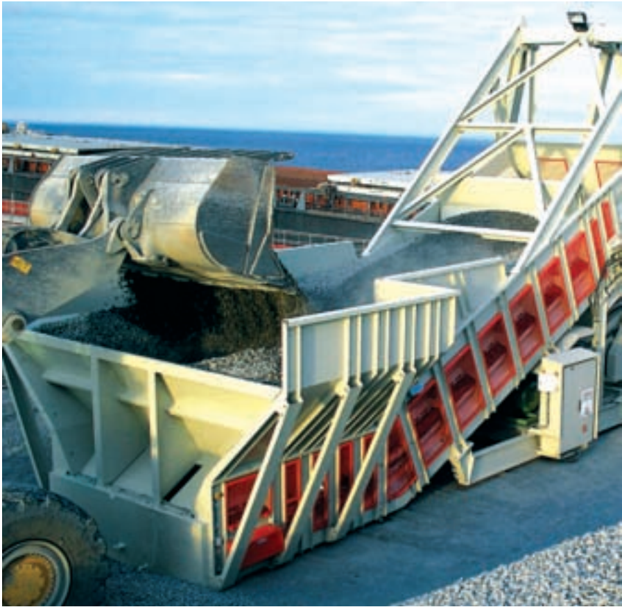
The Massive SAMSON™ 1600 receives Gabbros Rock from Shovels for Barge Loading at 1,000 t.p.h.
