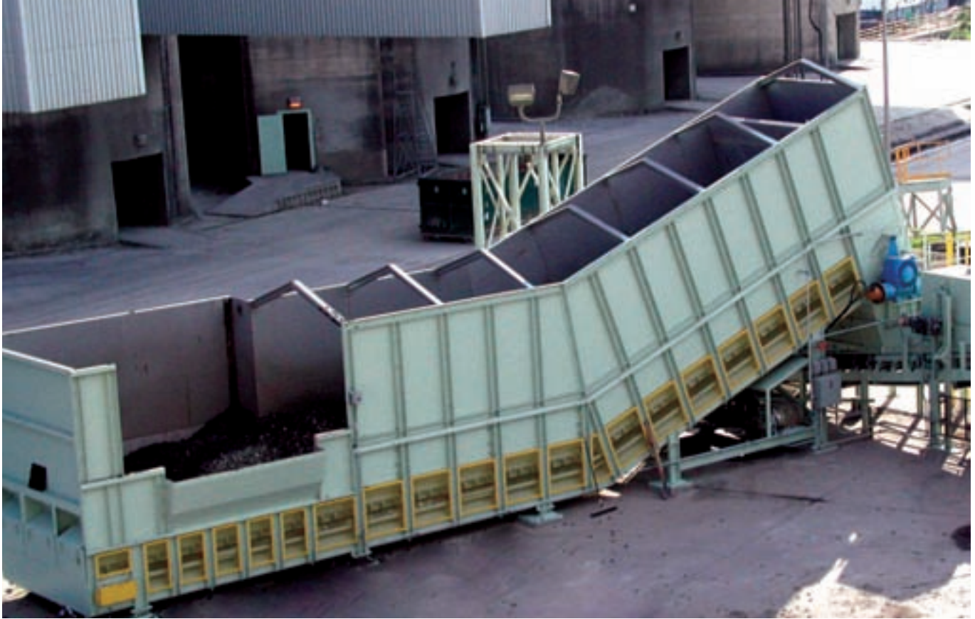
The SAMSON™ 800 Series provides 100 cubic metres of live storage for Alternative Fuels in a Cement Plant.
