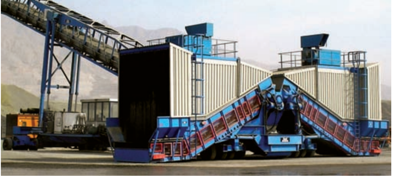
Twin SAMSON™ Feeders with Full Dust Control integrated to this Mobile Shiploader permits direct bulk export from Truck to Ship
