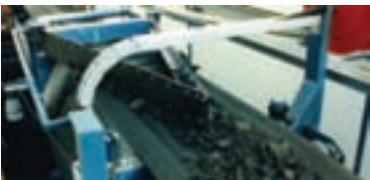
The SAMSON™ Horizontal Storage Bunker with Overhead Conveyor and Plough Discharger
