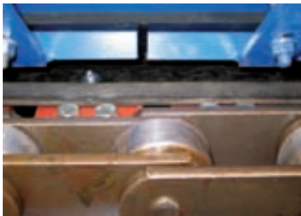
Load Carried on the Chain Rollers
