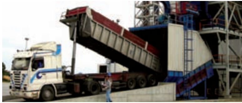
SAMSON™ Clinker Intake for Cement Grinding Plant with integrated Dust Extraction
