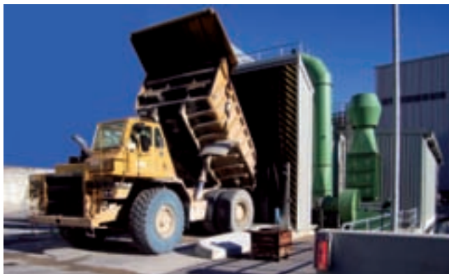
Enclosure with Extended Flared Entry for large Mining Dump Trucks
