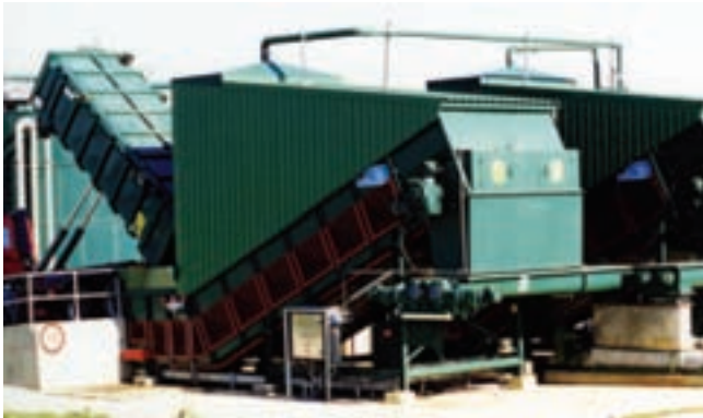
Enclosure with Fume Extraction for Odious Materials
