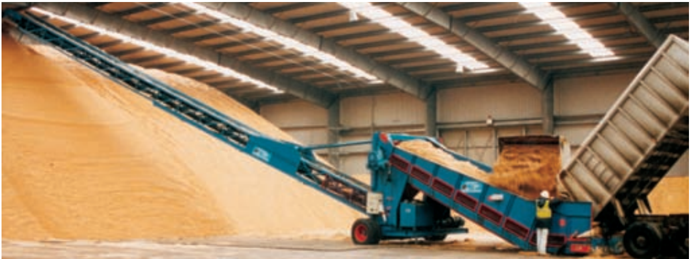
STORMAJOR™ combines the benefits of a SAMSON™ Surface Feeder with a Radial Stacking Boom mounted to a Common Mobile Chassis
