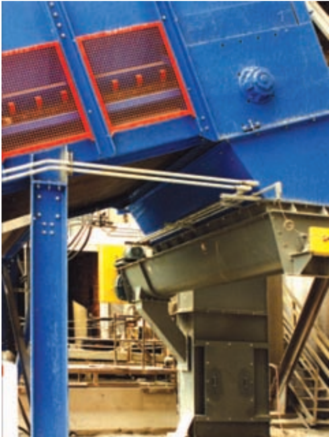
Single Screw Feeder provides metered output to a Bucket Elevator
