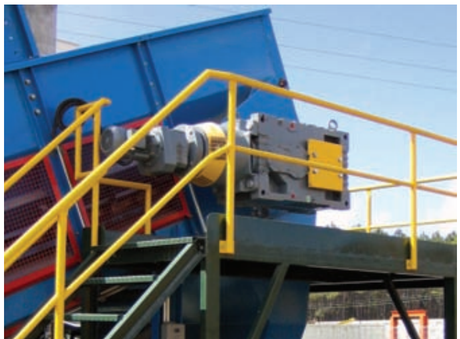
High efficiency Helical/Bevel main reduction gear with helical primary
