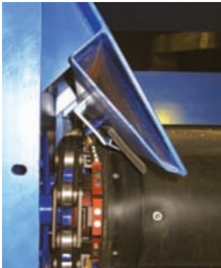
Flexible Side Seal with outer Belt Ledge
