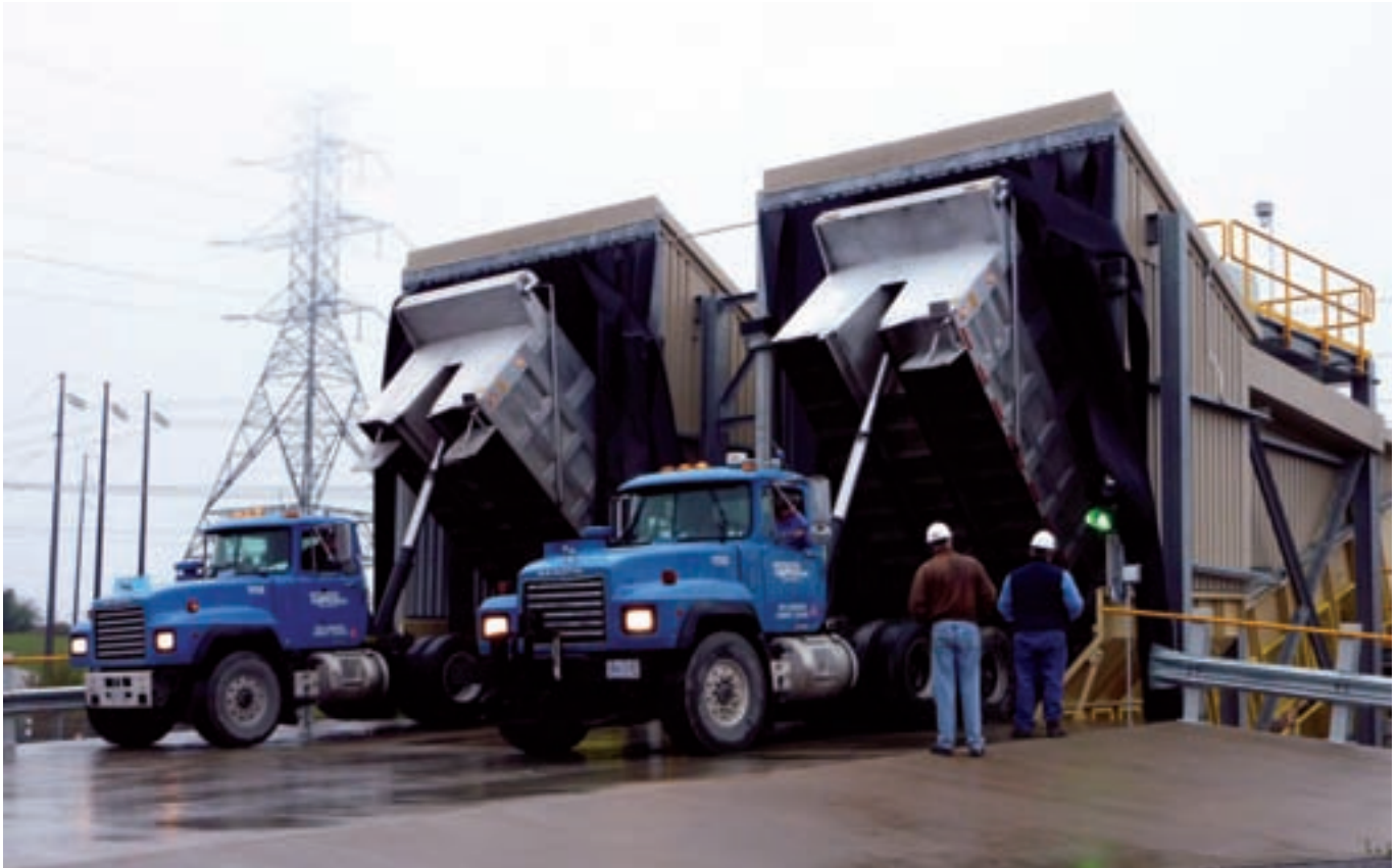
Twin SAMSON™ Surface Feeders receive minus 25 mm Limestone for the Flue Gas De-Sulphurisation system in a US Power Plant
