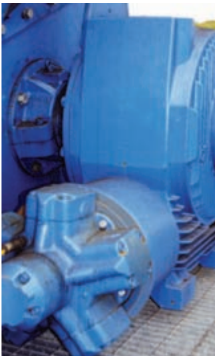
Direct Coupled Hydraulic Motor Drive with local or remote hydraulic power unit allowing the electric motor and control equipment to be positioned clear of the feeder in a more accessible location
