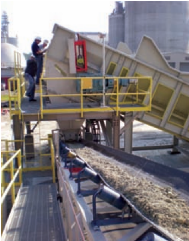
SAMSON™ 1600 with Tandem Drives using two Helical/Bevel Speed Reducers mounted one each side of the extended head shaft
