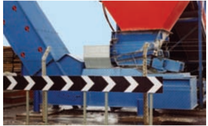
Vibro-Feeder controlling feed rate to a Steep Angle Belt Conveyor
