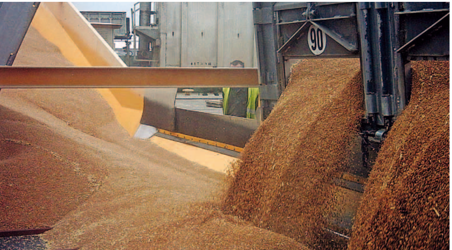
Independent Multi-Tip Samson™ with extended entry section to permit four trucks to discharge simultaneously
